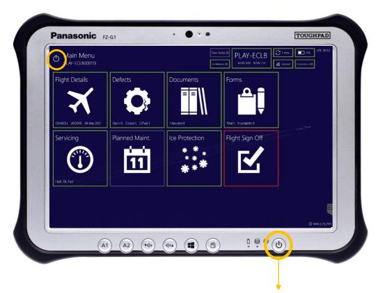
**NOTE:** Please do **NOT** use the *Power Switch* button on the device for regular shut down
